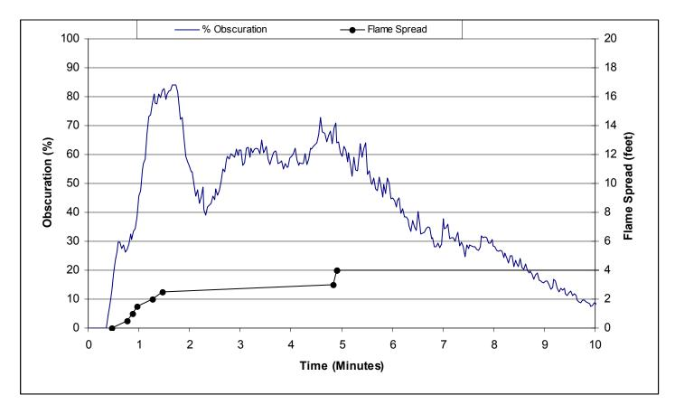
Test No. 1 07CA56359 / SV17122 12030712 Flame Spread Index: 15 Smoke Developed Index: 450 Max. Flame Spread: 4.0
